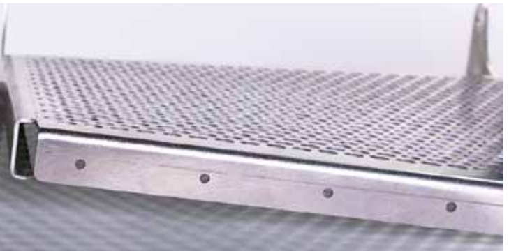
RIGHT PHOTOS: Original part resulted in extreme warpage and oil canning
